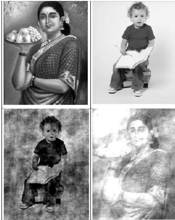
(a) test image1 (b) test image2 (c) Image Reconstruction from Magnitude of Image1 and Phase of Image2 (d) Image Reconstruction from Magnitude of Image2 and Phase of Image1
